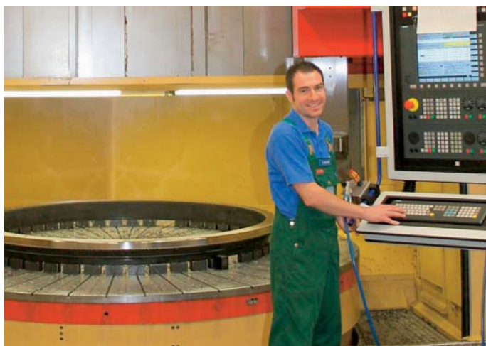
A new metal working lathe prepares rings for the bearings.
