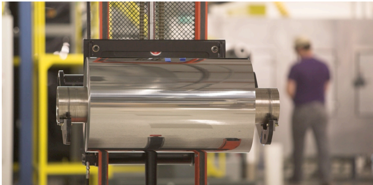
Figure 3: Nanosolar uses a proprietary low-cost alloy of highly conductive, wide-web aluminum foil.
